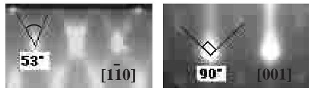
**Fig. 3.** Details of RHEED patterns along the [001] and [1 $\bar{1}0$ ] azimuths of 50 Å DyFe<sub>2</sub>(110) grown at 550 °C.
